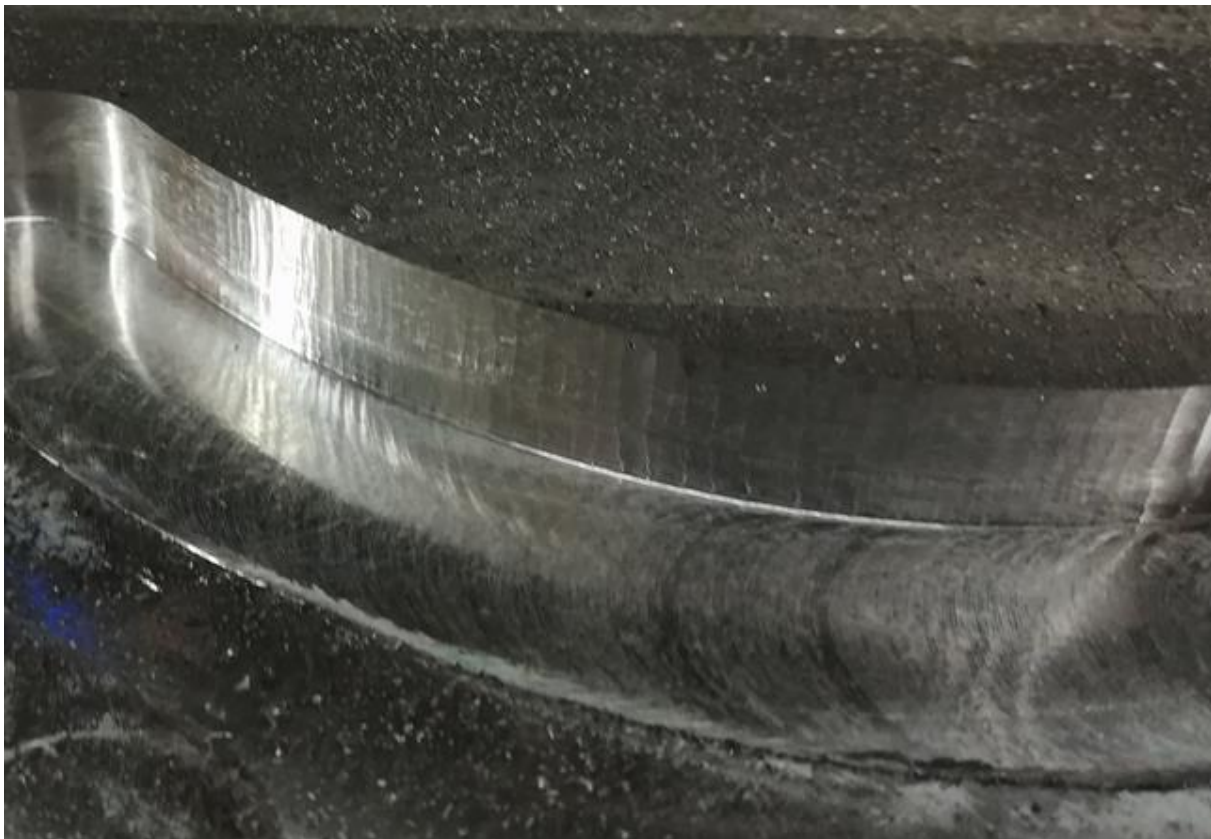
Figure 5. Chatter marks both on the vertical and horizontal surfaces of a workpiece.
