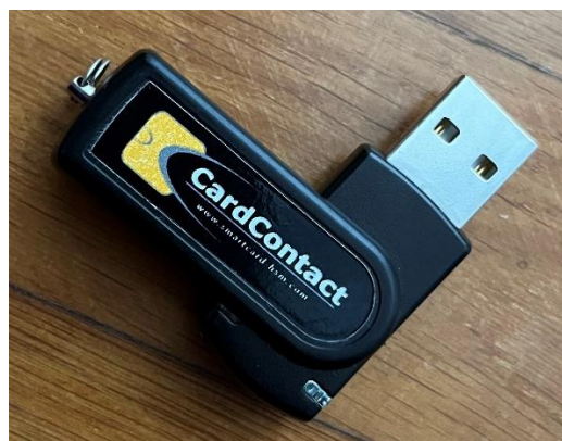
Figure 8. CardContact USB-Token HSM used in the project
